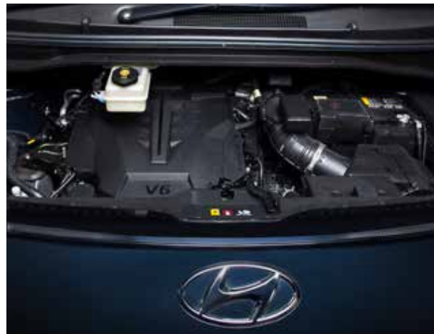
V6 λ III 3.5 MPI engine
